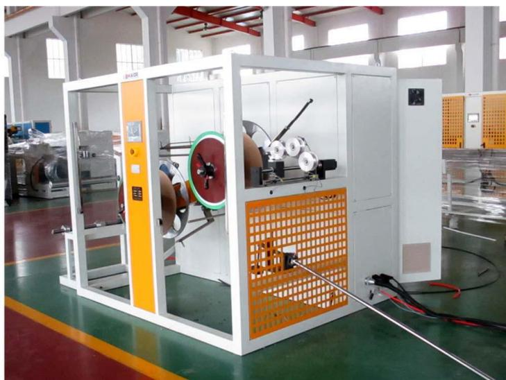
◎ Automatic winding machine is driven by servo motor and controlled by SIEMENS PLC system.
