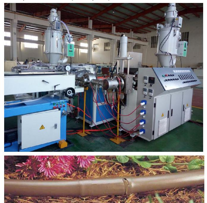
© The outer layer thickness is take about 10%-15%, very thin. And certain percent of recyced raw materials can mixed into the inner layer for saving cost.
