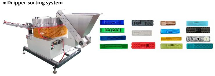
Most advanced detecting technologies are applied, such as nanoscale laser identifying device and dripper anti-direction rejecting device, ensuring drippers in production are 100% qualified.
