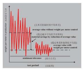
High precise Gravimeter control system of is applied in this PPR pipe production line. © It is used for measuring & calculating and precise control of pipe weight per meter and its extrusion output, to realize the constancy of pipe weight.
